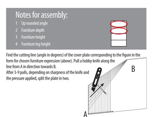
HINT: If necessary, place some paint tape on the front side where the split occurs, to reduce the risk of burs. Pull the knife towards yourself with a constant pressure on the blade. Use a hobby knife with a sharp, stable and short blade.
