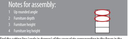
Find the cutting line (angle in degrees) of the cover plate corresponding to the figure in the form for chosen furniture expression (above). Pull a hobby knife along the line from A in direction towards B. R After 3-9 pulls, depending on sharpness of the knife and the pressure applied, split the plate in two.
